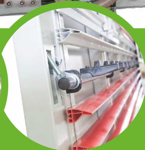
Tilting device for supporting small pieces to be cut
