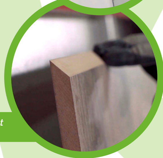
V-Grooving 90° on composite panels (Optional)
