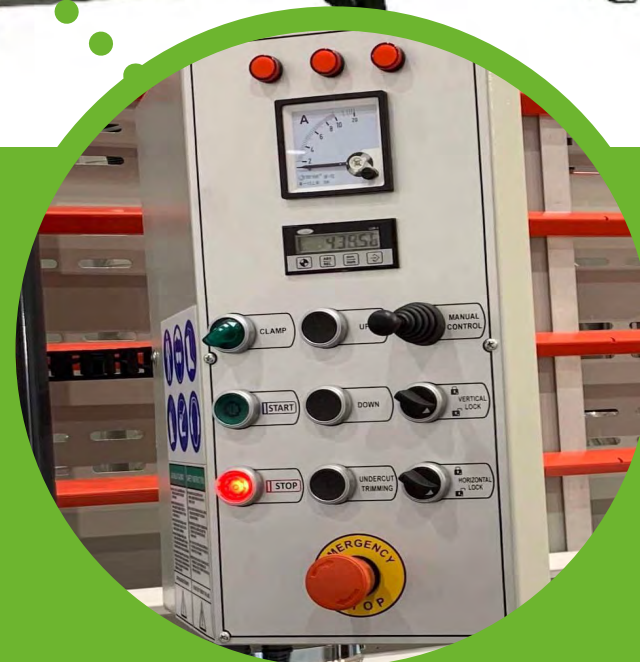
Pliers system for locking and moving panels with control board. Digital display included for the perfect adjustment of cuts in vertical and horizontal.
