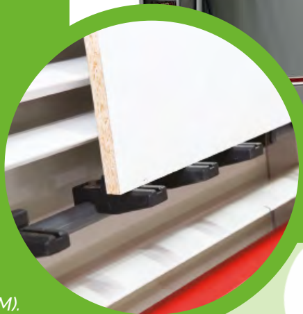
Tilting device for supporting the small pieces to be cut
