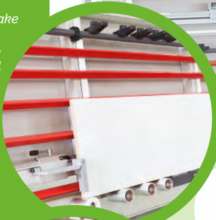
Lower supports with metal wheels for panel support
