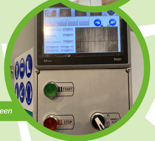
Digital display for the perfect adjustment of cuts in vertical and horizontal
