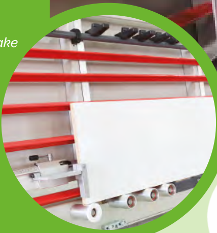
Lower supports with metal wheels for panel support
