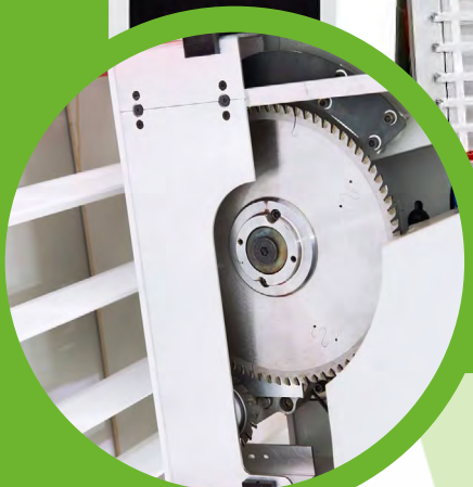
Turnable head for vertical and horizontal cuts
