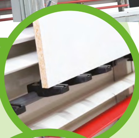
Tilting device for supporting small pieces to be cut
