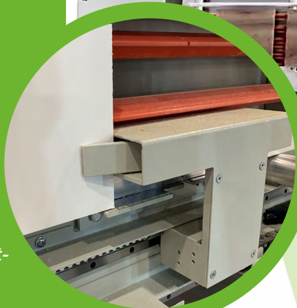
Horizontal pusher for cutting small panels vertically
