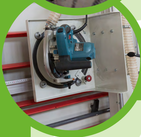
45° inclined cut on panel edge
