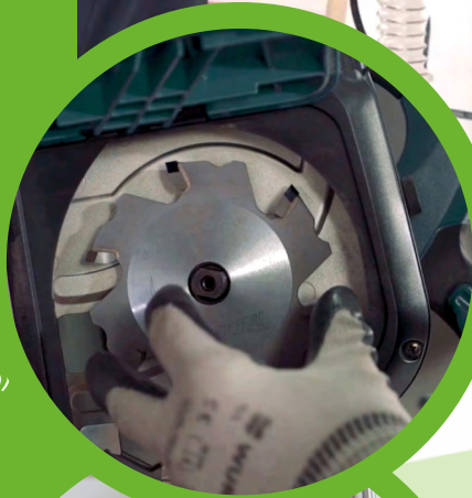
V-Grooving kit on composite panels (Optional)
