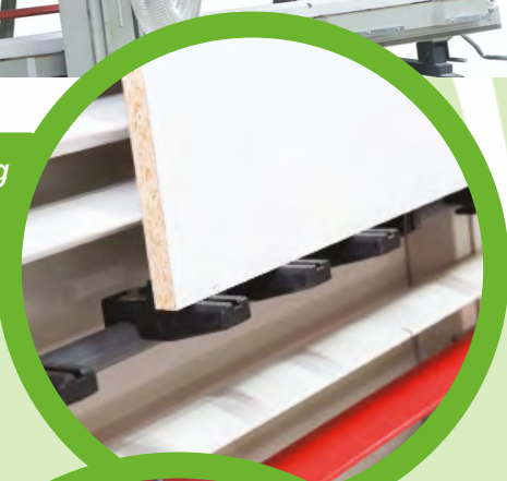
Tilting device for supporting small pieces to be cut
