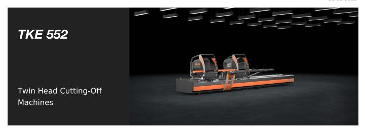
Twin-head cutting-off machine with automatic mobile head movement driven by an NC-controlled brushless motor. Pneumatic tilting of cutting units from 90° to 22°30′ (outward) in two fixed positions or with optional mechanical adjustment system for intermediate angles. Hydro-pneumatic blade feed.
