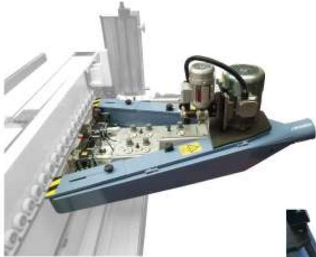
BELT SCHUUR UNIT
